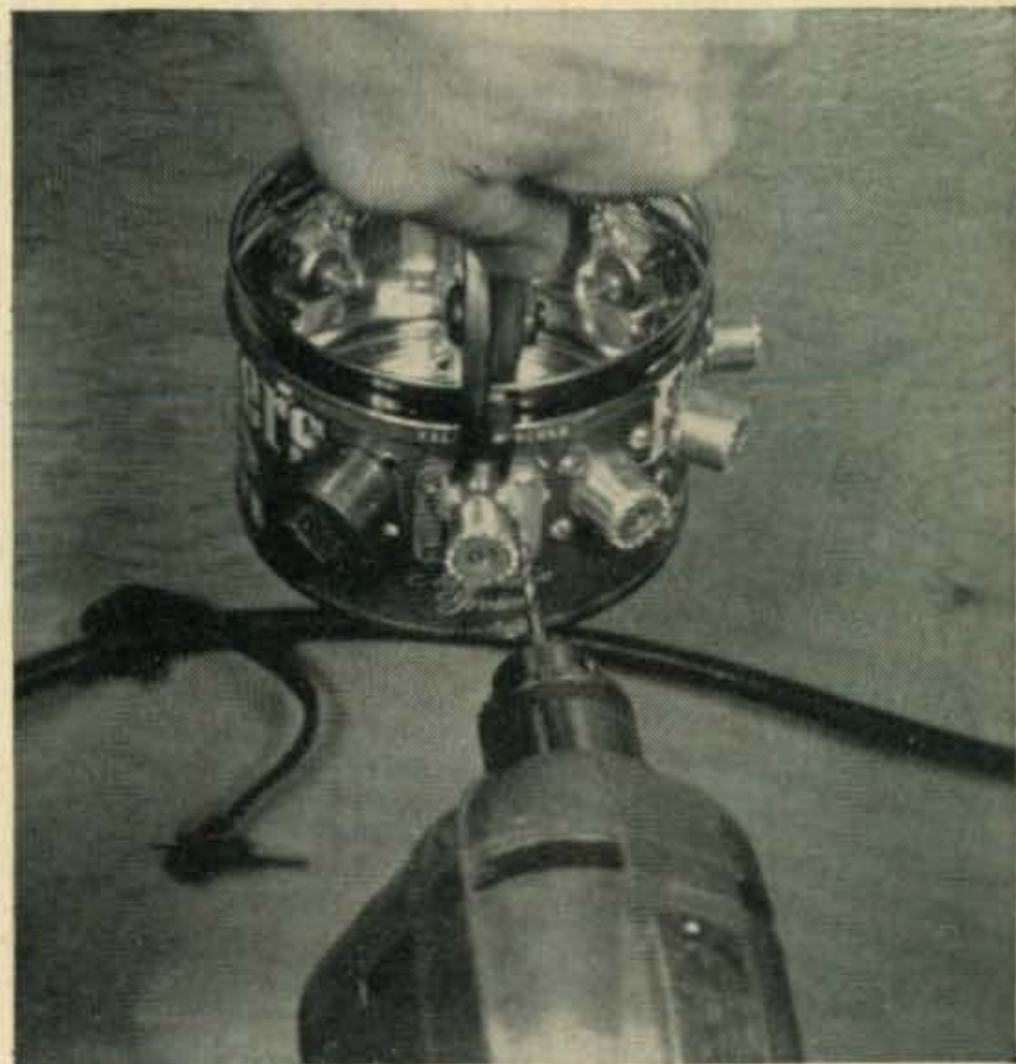
Fig. 2—Hold coax jack in place with pliers and drill the four mounting holes for 4-40 screws.
